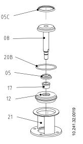
See section 9.9. Exploded drawing and parts list of the INNOVA M single seat valve and 9.10. Exploded drawing and parts list of the INNOVA L single seat valve for a reference to the parts described.
